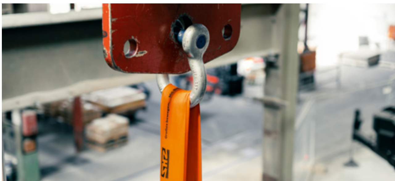
Combination shackle with heavy duty round sling
