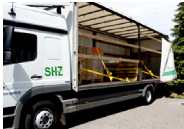
Combination of head lashing and tie-down lashing
